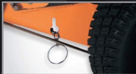
SWZ: De clutch cold-start feature enhances cold weather starting. It uses a large, easy-to-pull chain that locks into a slot in the engine deck to relieve pump pressure.
