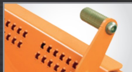
Foot pedal cutter deck lift is spring-assisted and makes raising the cutter deck smooth and easy.
