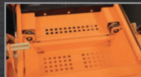
Pierced, extruded steel footplate is rubber iso-mounted for enhanced comfort.
